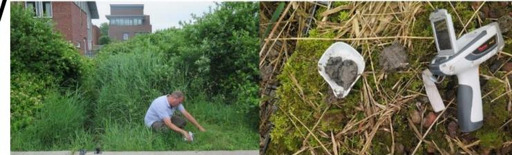
Soil sample at inlet - top soil for lab analysis
